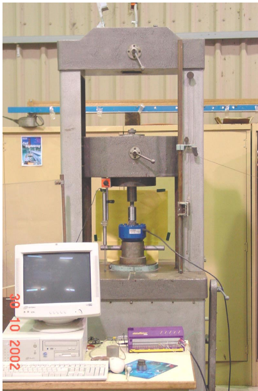
FIG.2a - Short Encapsulation test arrangement in a compression machine
